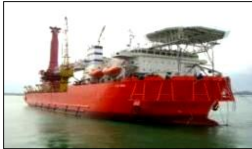
LTS 3000 DLB 3,000MT crane, 200MT tension, self propelled
