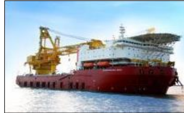
SapuraKencana 3500 DP-3 HLV 3,500MT crane, 390MT tension S-lay
