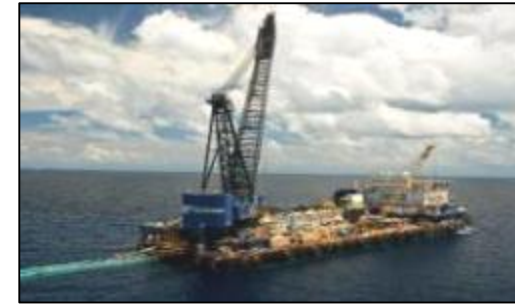
SapuraKencana 900 DLB 9,00MT crane, 120MT tension
