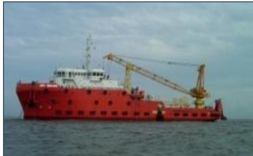
KPV REDANG 200 Pax Crane Capacity: 25T DP2
