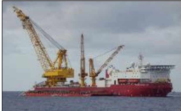
SapuraKencana 1200 DP-3 HLV 1,200MT crane, 520MT tension S-lay
