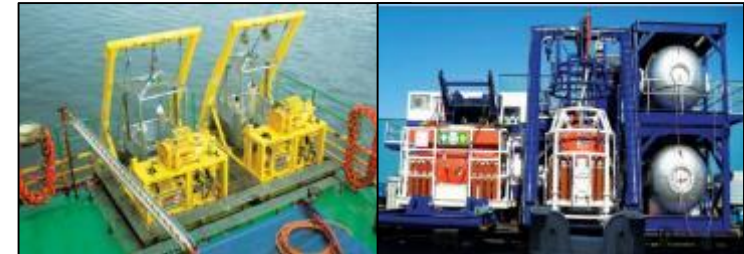
10 x Air dive system 4 x portable sat system 1x Hyperbaric Rescue Facility (HRF)
