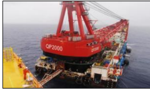
SapuraKencana 2000 DLB 2,000MT crane, 140MT tension
