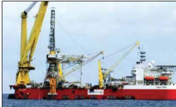
Sapura 3000 DP-2 HLV 2,722MT crane, 240MT tension S-lay, 400MT tension J-lay, 360MT A&R and A-frame capacity
